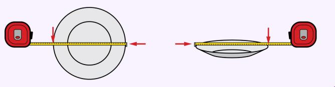
**COVER DIAMETER:** Place the plate cover top-side-down. Measure across full diameter of the plate cover with a tape measure, pulling to create slight tension on the tape measure. Make note of the exact measurement shown.
